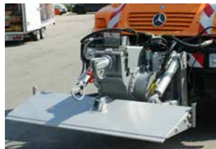
Top: Hydraulic front-mounted cable winch with 12 tractive force, wireless remote control and stabilisers on a Unimog truck.
